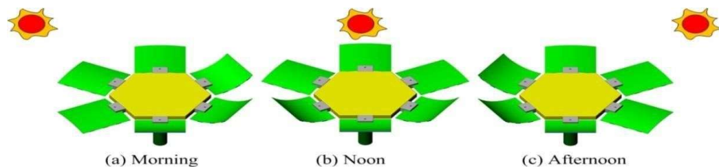
Fig 3: Application of bimetallic and laminate for solar tracking
