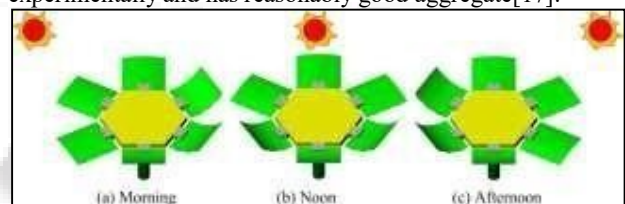
Fig. 7: Application of bimetallic and laminate for solar tracking
